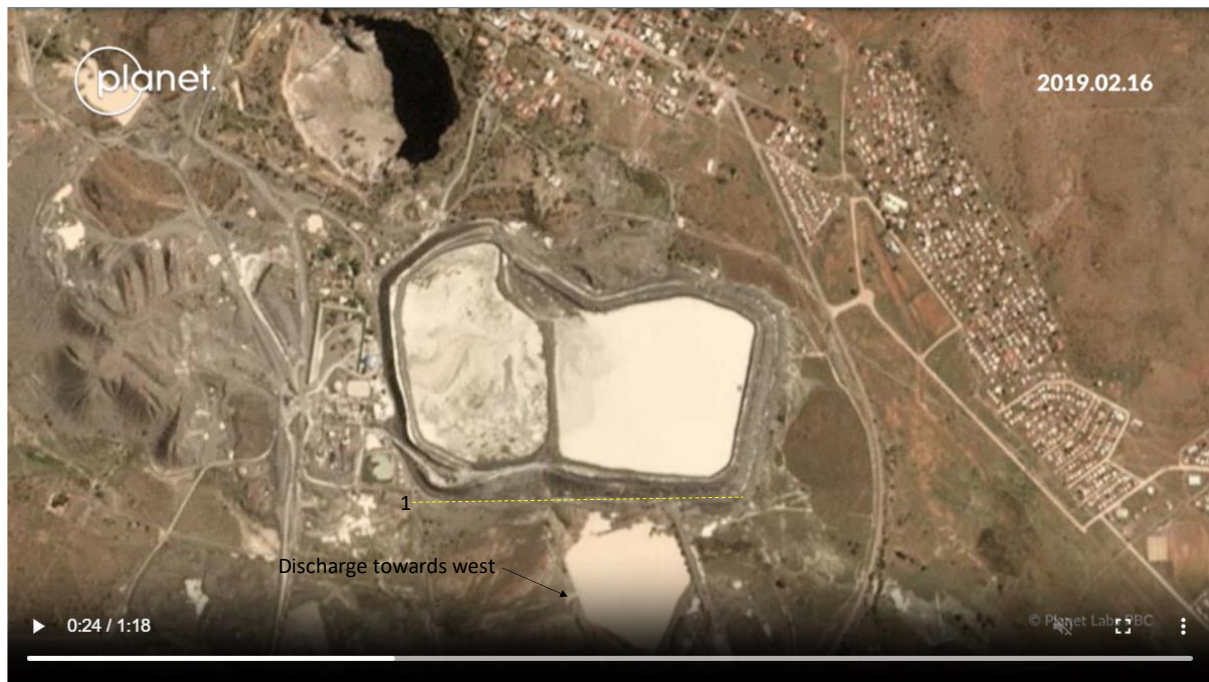
FIGURE 2 PLANETSCOPE SATELLITE IMAGES TAKEN ON 2019/02/16 SHOWING WATER DISCHARGING FROM DAM 10, UPSTREAM TOWARDS THE WEST, SUGGESTION THAT WATER IN DAM IS DID NOT ORIGINATE FROM NATURAL RUN-OFF.
