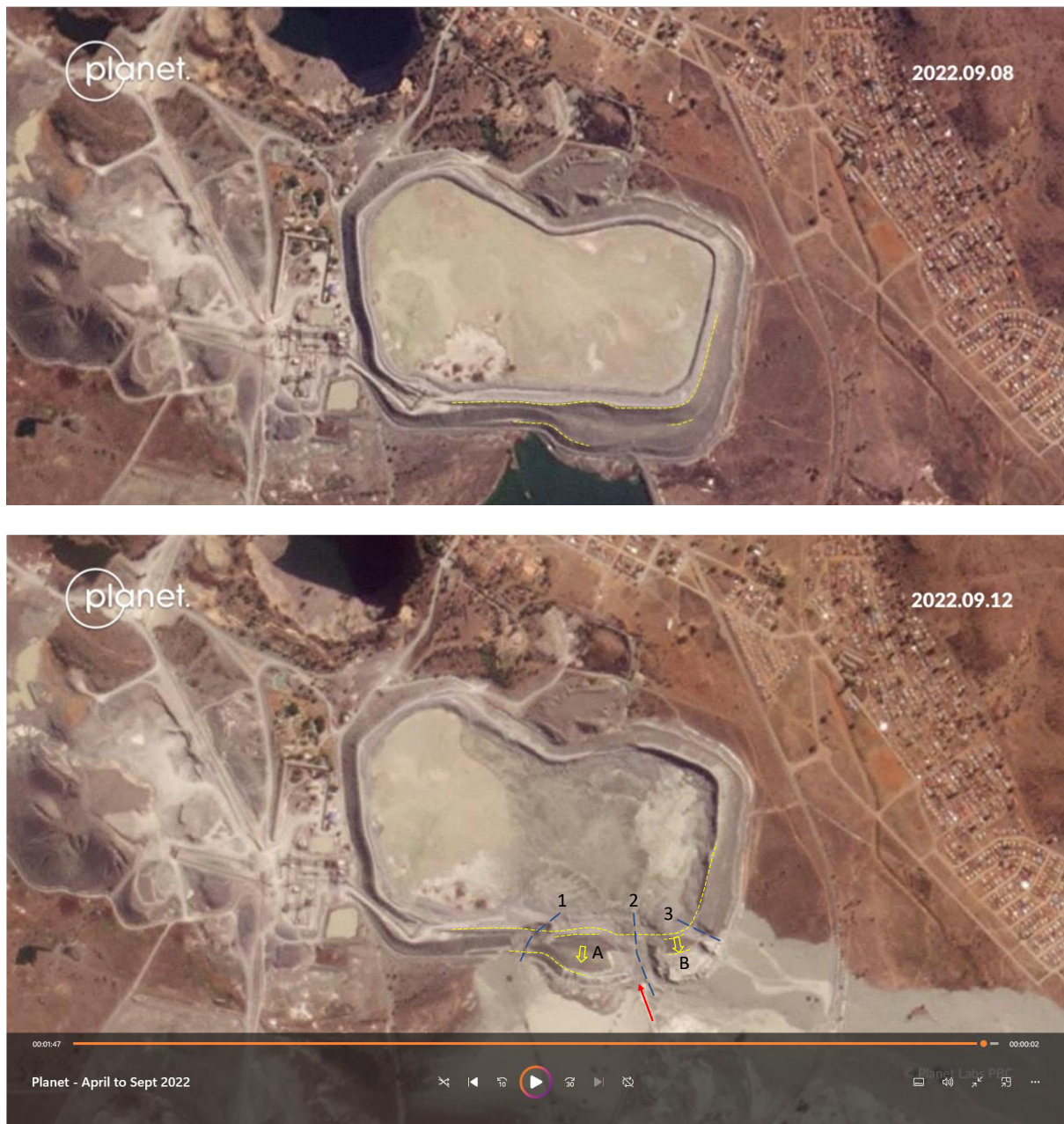
FIGURE 15 PLANETSCOPE SATELLITE IMAGES TAKEN BEFORE (2022/09/08) AND AFTER (2022/09/12) THE FAILURE EVENT
