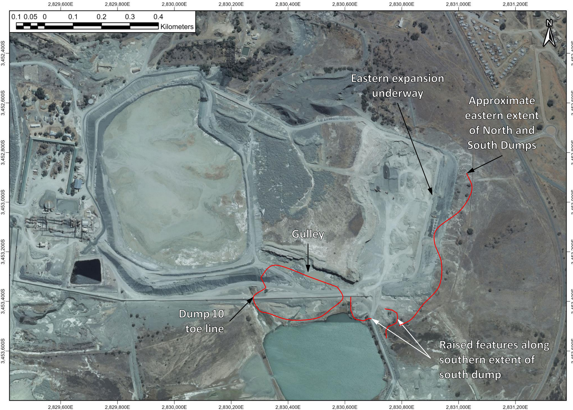
Figure B6: 2015-08-13 aerial image showing the alignment of a conveyor belt and the extent of the historic dumps.
