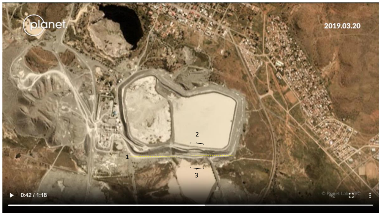
FIGURE 5 PLANETSCOPE SATELLITE IMAGE TAKEN ON 2019/03/20 SHOWING MOVEMENT ALONG THE TOE OF THE SOUTHERN WALL OF COMPARTMENT 2.
