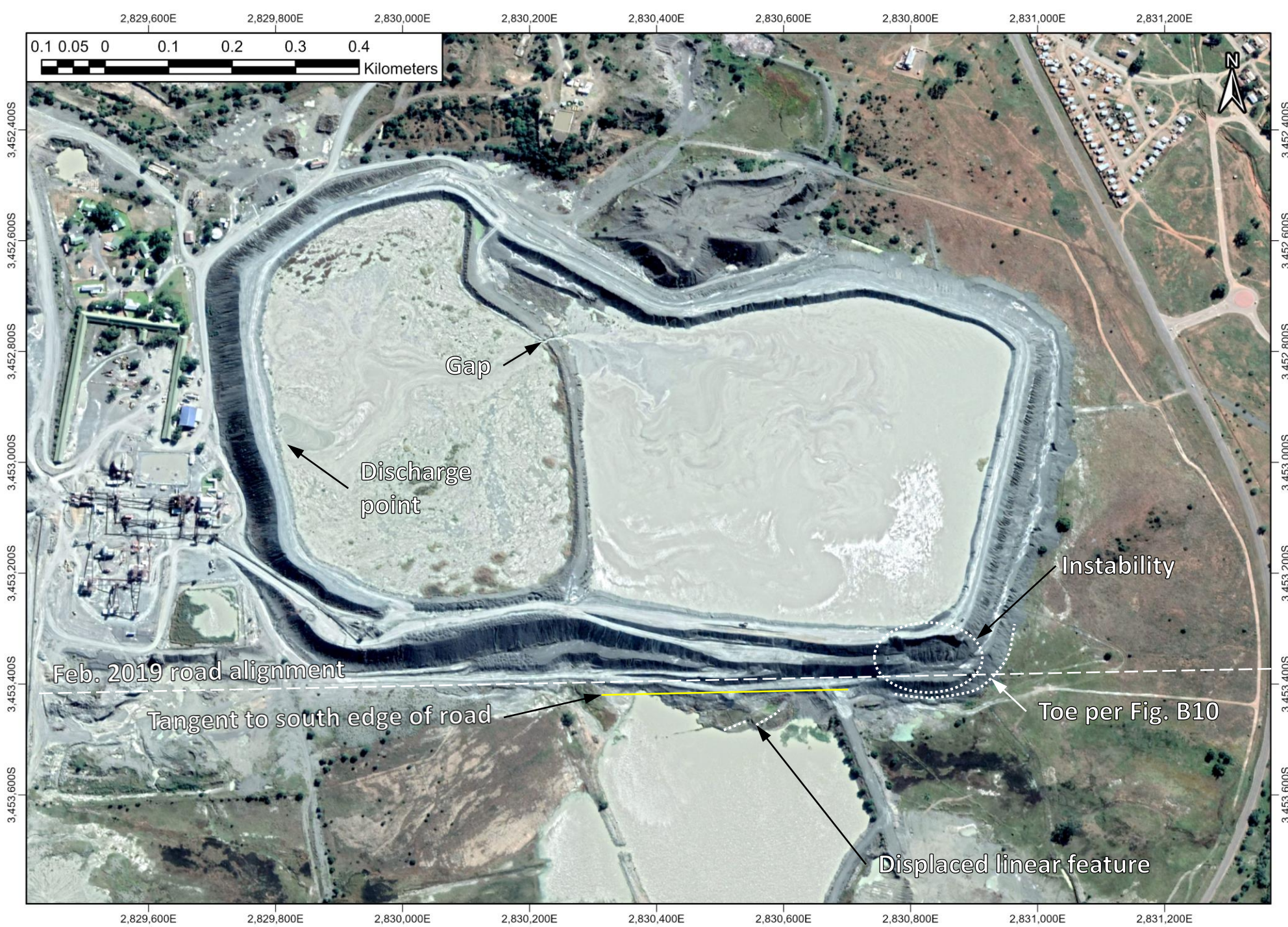
Figure B12: 2019-05-02 WorldView 2 satellite image highlighting the separation between the February 2019 (Figure B10) and the current location of the southern edge of the southern access road.
