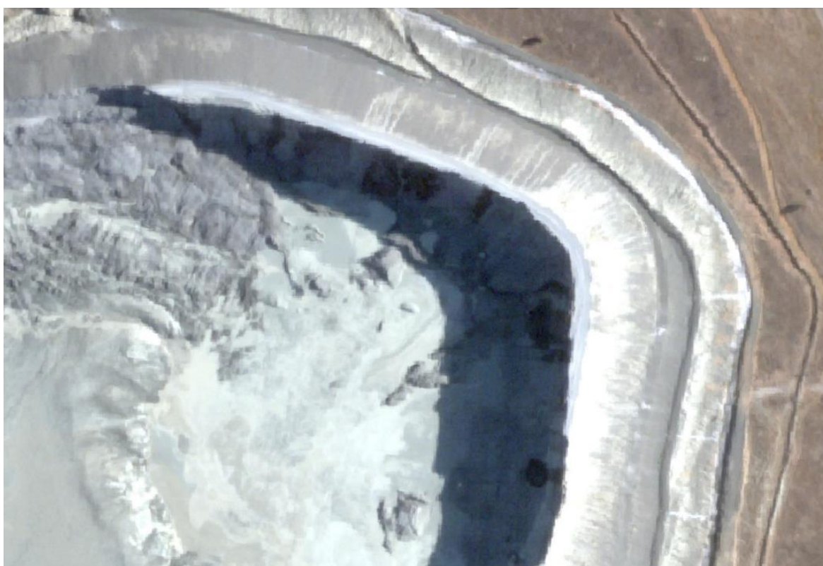
FIGURE 36 THE NORTH-EASTERN PART OF THE TAILINGS DAM BEFORE AND AFTER FAILURE (26 JULY 2022 AND 12 SEPT 2022 RESPECTIVELY). THE WHITE STREAKS ON THE NORTHERN AND EASTERN SLOPES VISIBLE ON THE POST-FAILURE IMAGE SUGGEST THAT LIMITED OVERTOPPING MAY HAVE OCCURRED AT THESE LOCATIONS.
