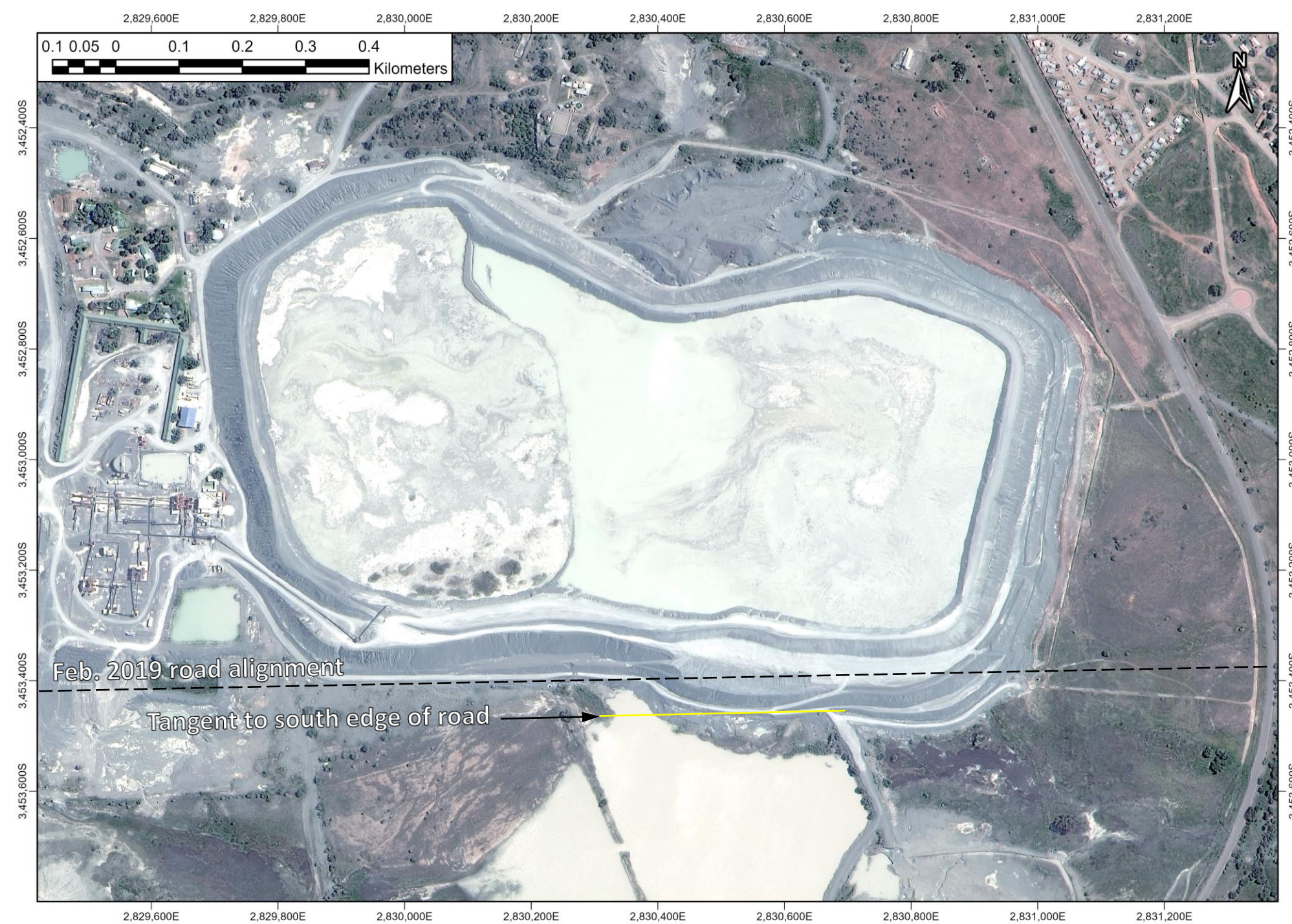
Figure B19: 2021-02-17 SuperView satellite image highlighting the separation between the February 2019 (Figure B10) and the current location of the southern edge of the southern access road.
