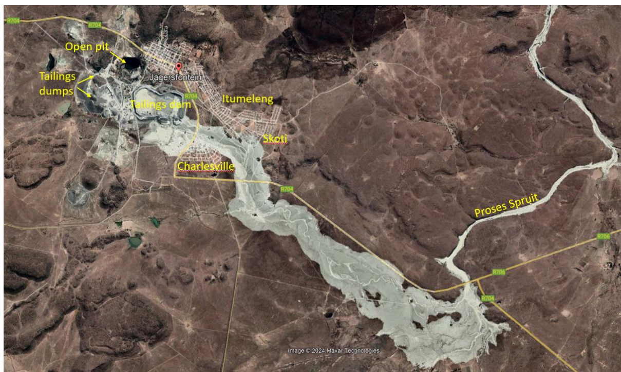
FIGURE 2 LOCALITY PLAN SHOWING THE TOWN OF JAGERSFONTEIN AND SOME OF THE EXTENT OF THE IMPACT FORM THE FAILURE (GOOGLE EARTH). IMAGE DATED 16 SEPTEMBER 2022.
