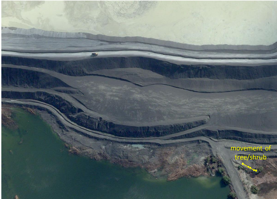
FIGURE 11 “THE WANDERING TREE”: MOVEMENT OF A TREE OR LARGE SHRUB TRACKED NEAR THE NORTHERN END OF THE DAM 10 EMBANKMENT FROM SATELLITE IMAGES DATED 9 JULY 2020 TO 28 JULY 2022 (FIGURES B15 TO B22) (TOTAL EXTENT OF MOVEMENT WAS 28 M).
