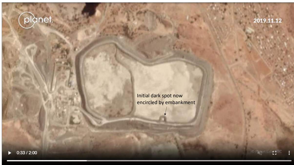
FIGURE 9 PLANETSCOPE IMAGING DATED (A) 2019/09/16 AND (B) 2019/11/12 SHOWING A DARK SPOT APPEARING ALONG SOUTHERN EMBANKMENT, SUBSEQUENTLY ENCIRCLED BY EMBANKMENT.
