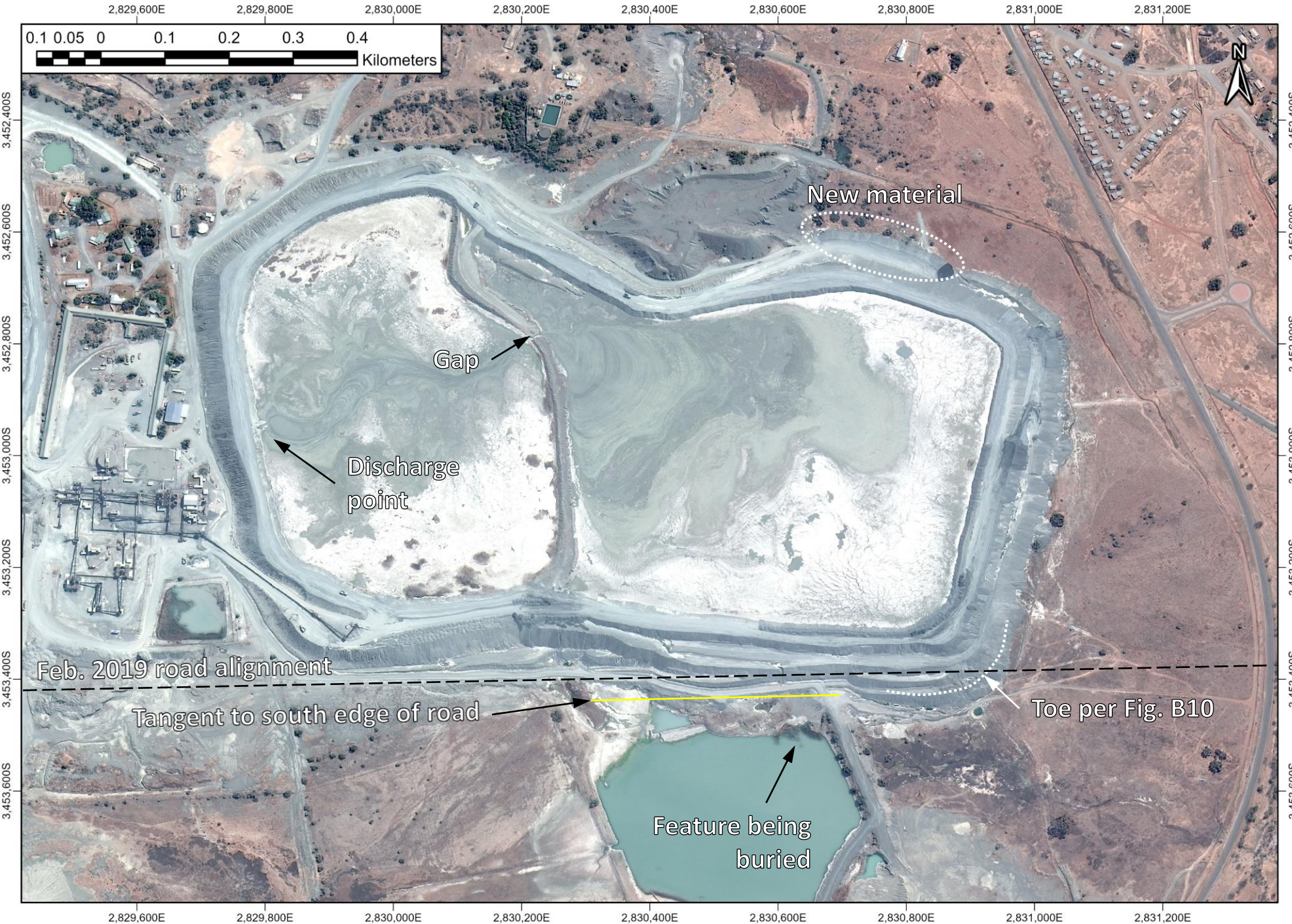
Figure B13: 2019-09-14 SuperView satellite image highlighting the separation between the February 2019 (Figure B10) and the current location of the southern edge of the southern access road.
