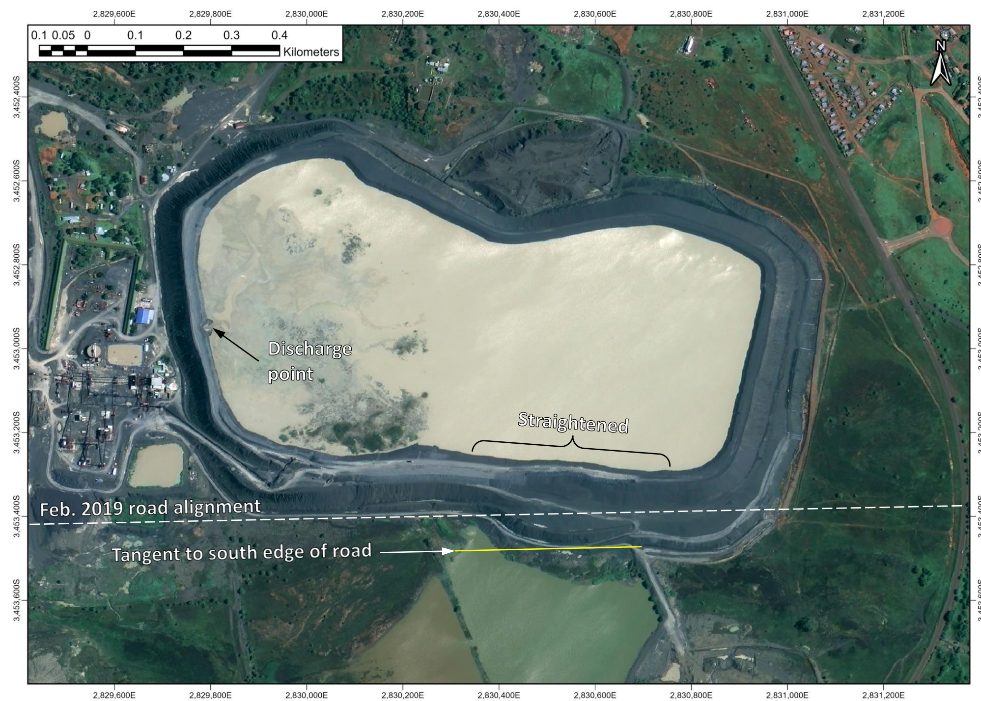
Figure B20: 2022-01-12 Jilin-1 satellite image highlighting the separation between the February 2019 (Figure B10) and the current location of the southern edge of the southern access road.
