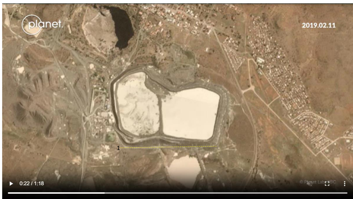
FIGURE 1 PLANETSCOPE SATELLITE IMAGES TAKEN ON 2019/02/07 AND 2022/02/11 SHOWING RAPID FILLING OF DAM 10.
